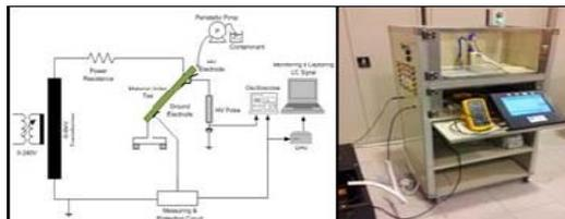
**Fig. 1:** Schematic diagram of Incline-Plane Tracking (IPT) test
