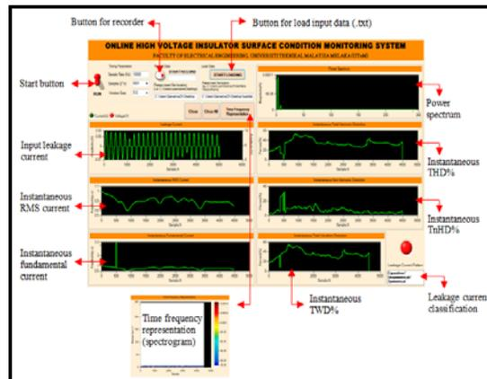
Fig. 2: Front panel of leakage current monitoring system
