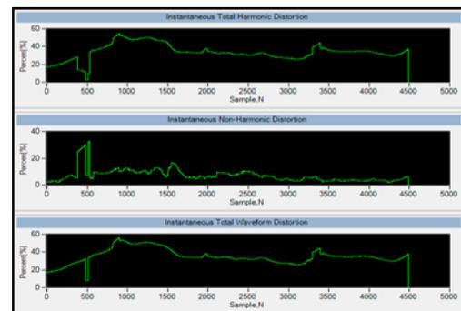
**Fig. 8:** Harmonic components for non-linear pattern
