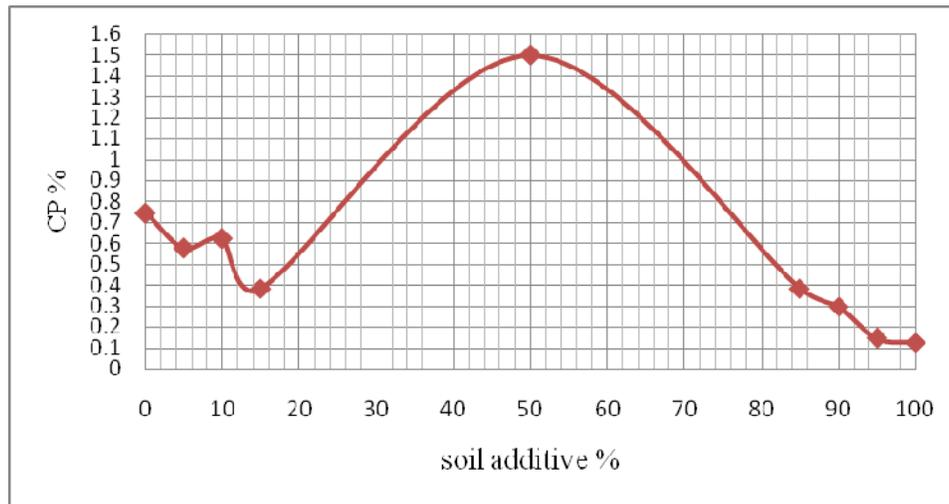
**Fig. 1:** variation (SM) soil content with collapse potential (CP) for mixture soil.
