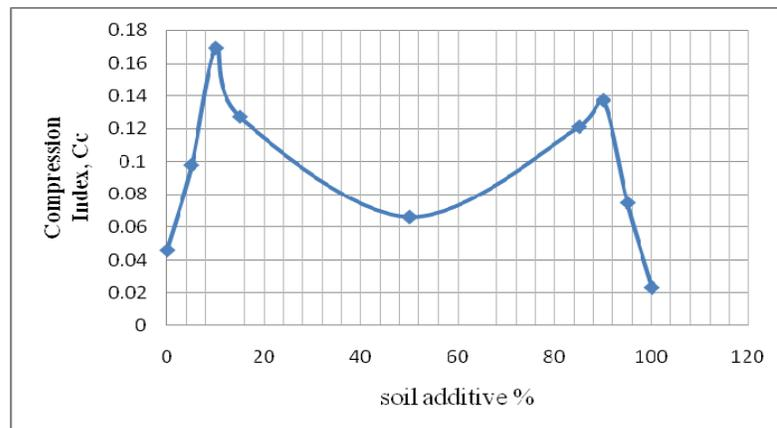
**Fig. 4:** variation (ML) soil content with compression index (Cc) for mixture soil.
