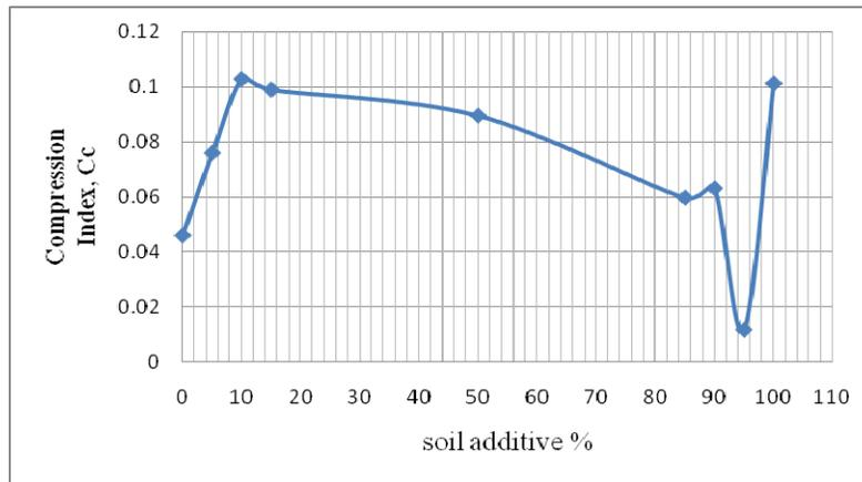
**Fig. 3:** variation (SM) soil content with compression index (Cc) for mixture soil.
