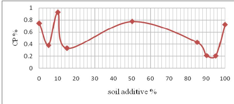
**Fig. 2:** variation (ML) soil content with collapse potential (CP) for mixture soil.
