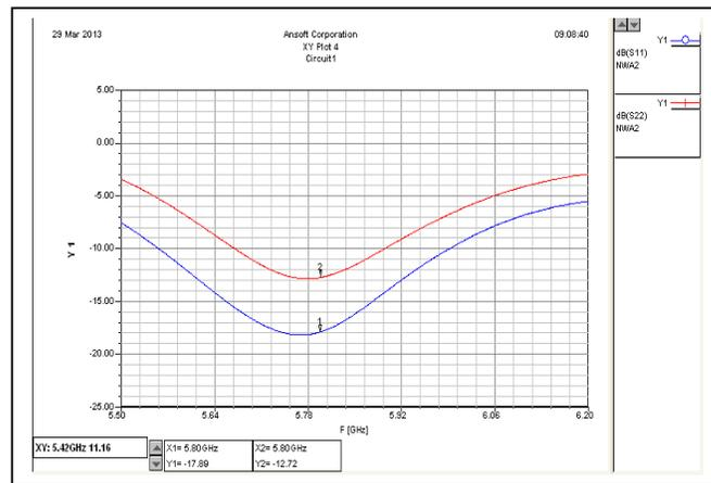
**Fig. 5(a):** Input Reflection Loss ( $S_{11}$ ) and Output Reflection Loss ( $S_{22}$ )
