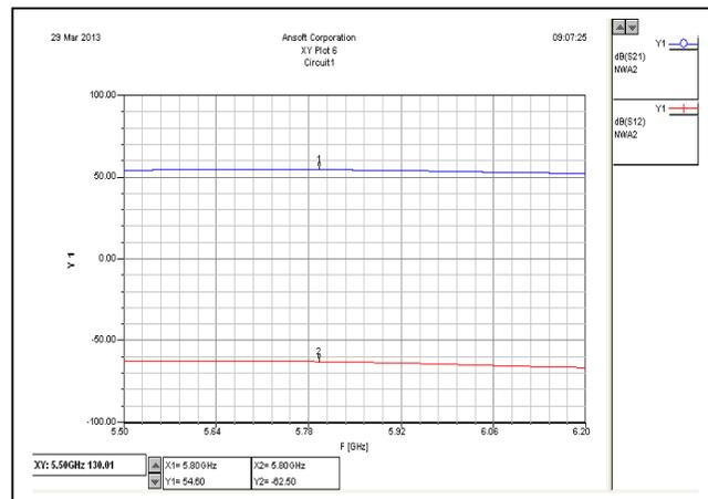
**Fig. 5(b):** Forward Transfer ( $S_{21}$ ) and Return Loss ( $S_{12}$ )
