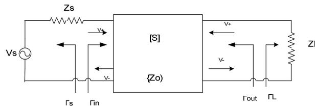
**Fig. 3:** I/O circuit of 2-port network [5]
