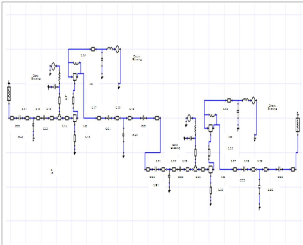
**Fig. 4:** Complete schematic double- stage Cascoded LNA
