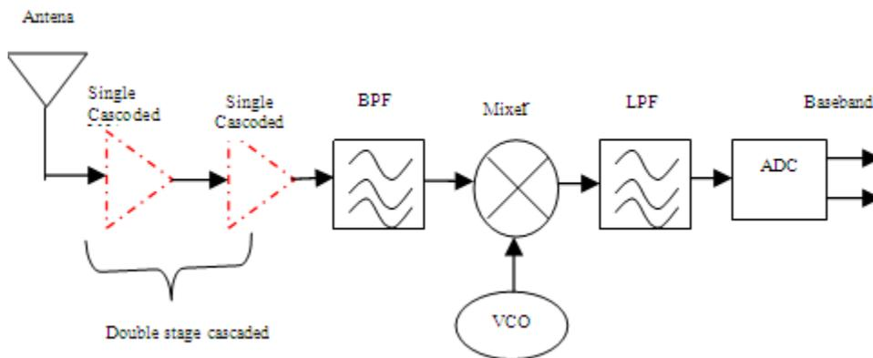
**Fig. 1:** Direct conversion RF front-end receiver using double stage cascaded LNA configuration
