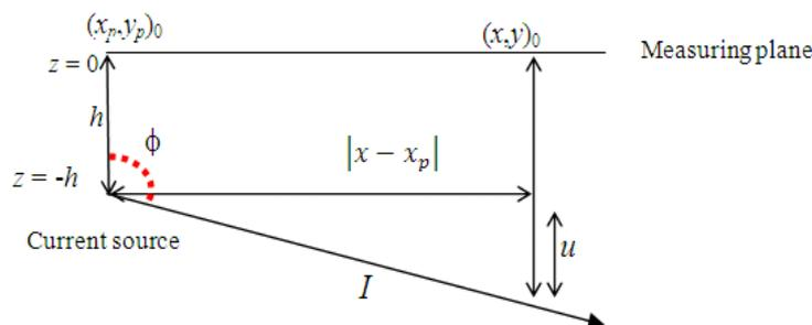
**Fig. 2:** The height of a measuring point from the flowing current (Yun, 2006).
