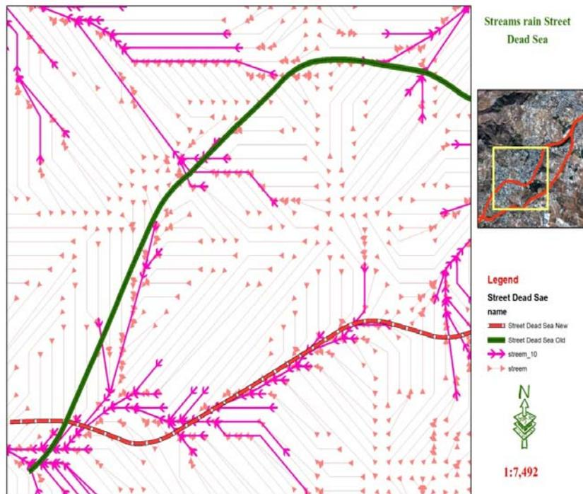
Fig. 8: The Drainage pattern for the area surrounding the Amman-Dead Sea highway.
