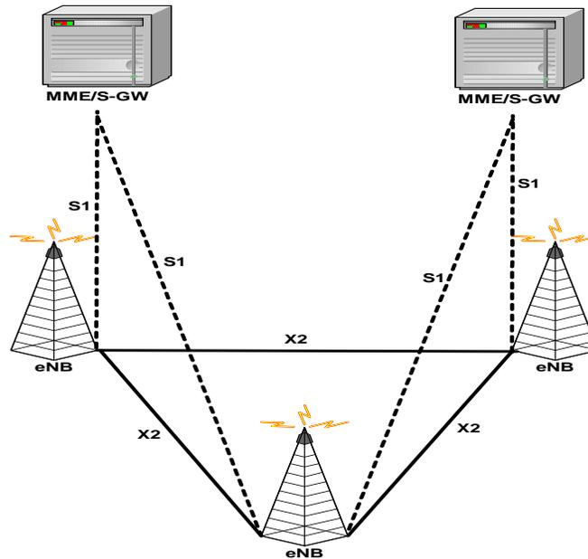
**Fig. 2:** LTE system architecture.
