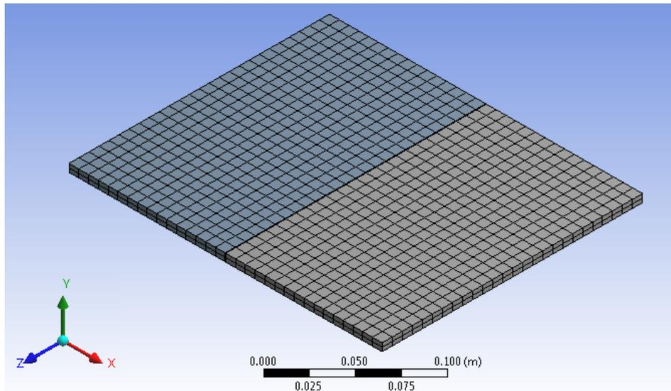
Fig. 3: Meshing of model.
