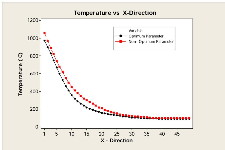
Fig. 4: Graph Comparison of temperature profile in the middle of the plate,  $z = 100$  mm.
