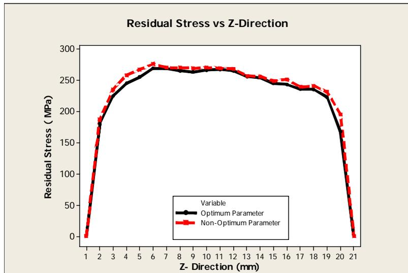
**Fig. 7:** Graph Residual Stress in  $z$  direction in the plate at mid span along the weld.
