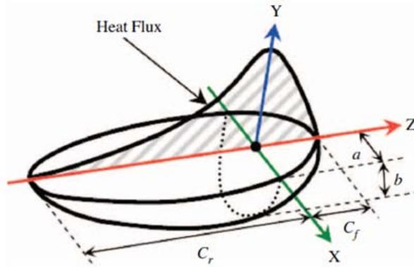
**Fig. 1:** Double ellipsoid heat source configurations.
