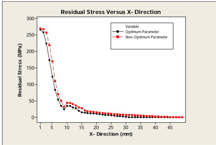
**Fig. 6:** Graph Residual Stress in  $x$  direction in the middle of the plate,  $z = 100$  mm.
