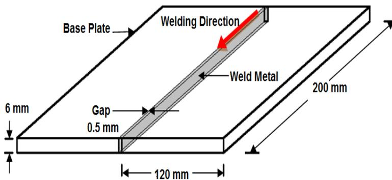
Fig. 2: Geometry of model.
