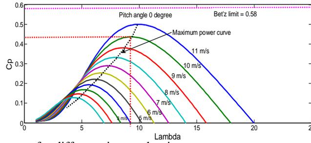
**Fig. 1:** Power co-efficient curve for different tip speed ratio.
