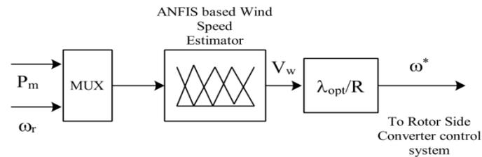
Fig. 4: ANFIS-based MPPT control module of turbine rotor speed.
