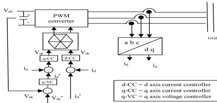
Fig. 3: Overall vector control of the GSC.
