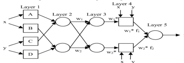
Fig. 5: Structure of ANFIS controller.
