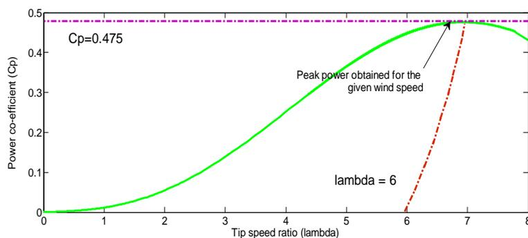
**Fig. 13:** Power co-efficient curve for different tip speed ratio obtained by proposed MPPT controller.
