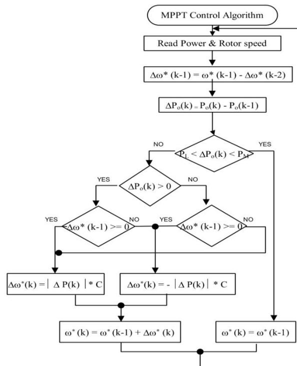
Fig. 6: Flow chart of MPPT controller.
