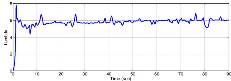
**Fig. 10:** Tip speed ratio of the WECS.
