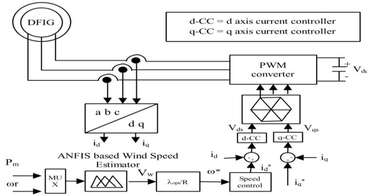
Fig. 2: Overall vector control of the RSC.
