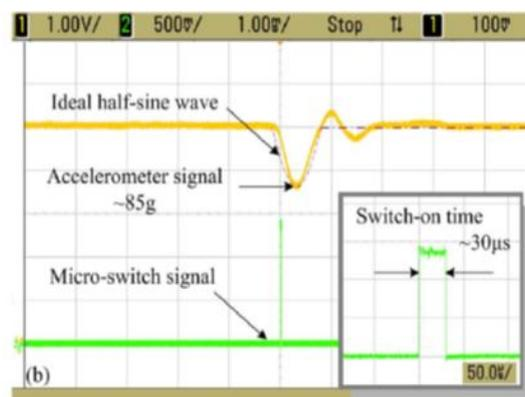
**Fig. 5:** Test result under 85g acceleration (HAOGANG, 2009)
