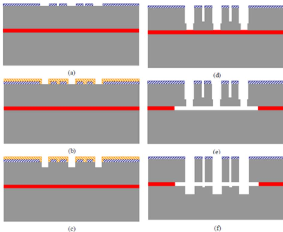
**Fig. 7:** Fabrication flow of dry release process (XU, 2009)
