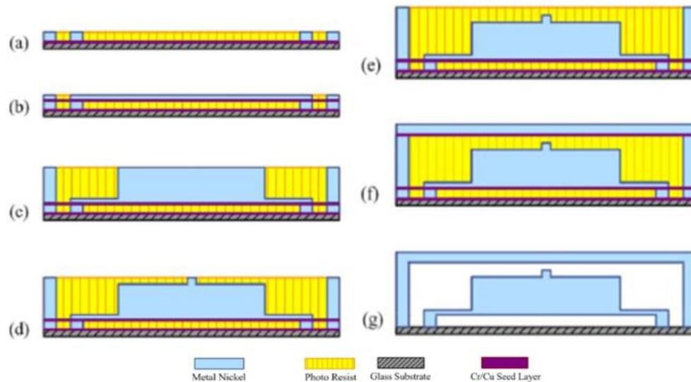
**Fig. 8:** Fabrication of Surface micromachining (Haogang, 2009)
