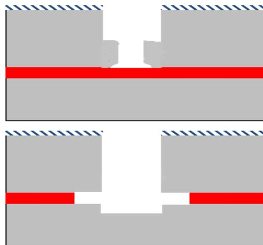
**Fig. 2:** Layout schematic before (top) a) and after (bottom) b) anti-footing method (Xu, 2009).
