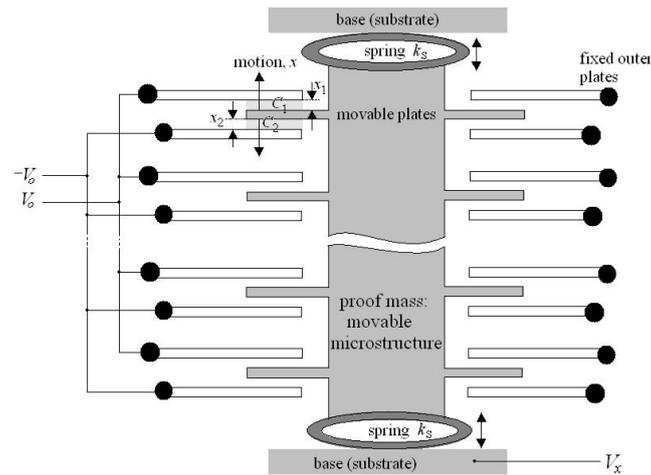
**Fig. 1:** Accelerometer structure. The springs ( $k_s$ : spring constant) is attached to proof mass at substrate where it moved up and down. From the movable and fixed plates, the capacitors is determined (Lyshevski, 2002)
