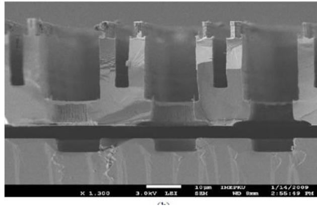
**Fig. 10:** Cross section view of SOI structure after final etching.
