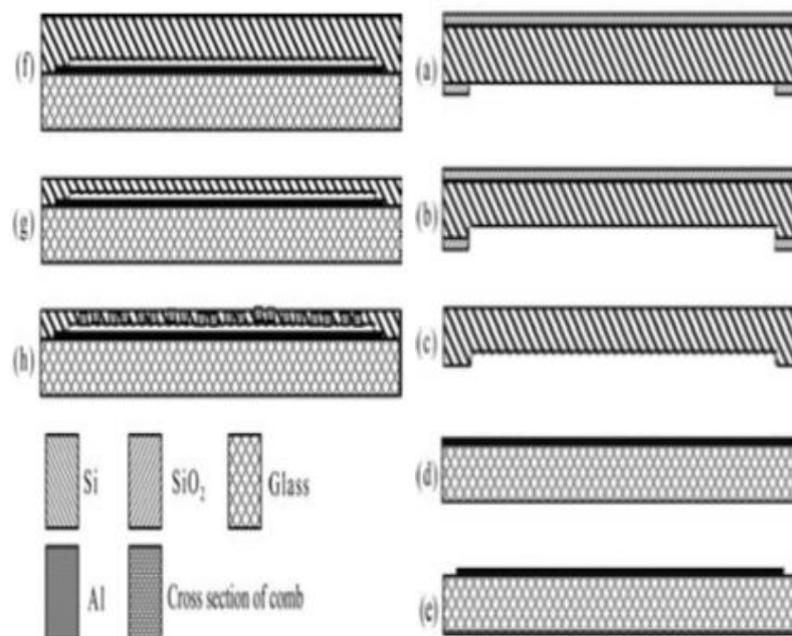
**Fig. 9:** Fabrication of two sided device using Bulk Micromachining (Dong Linxi, 2009)
