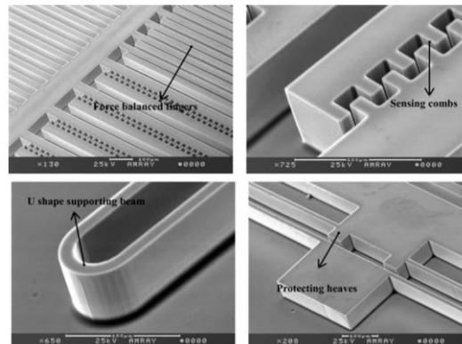
**Fig. 11:** SEM picture of the fabricated device.
