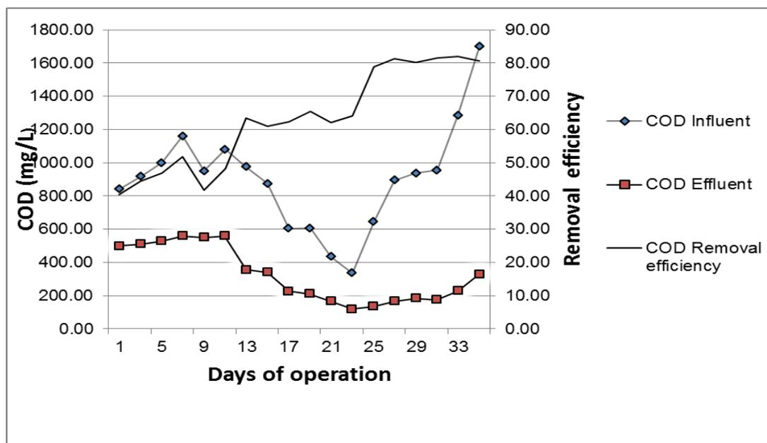
Fig. 2: COD removal efficiency of the HUASB reactor during start-up period.
