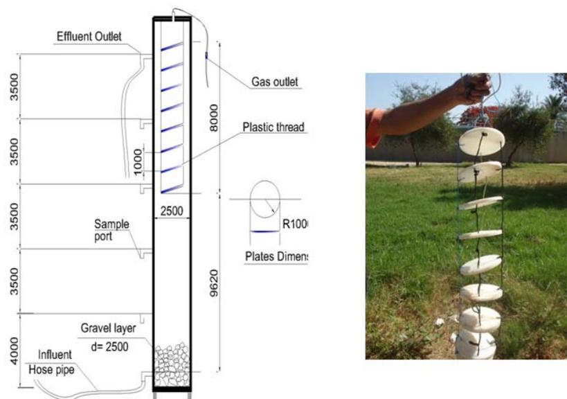
**Fig. 1:** Schematic diagram of the UASB reactor.
