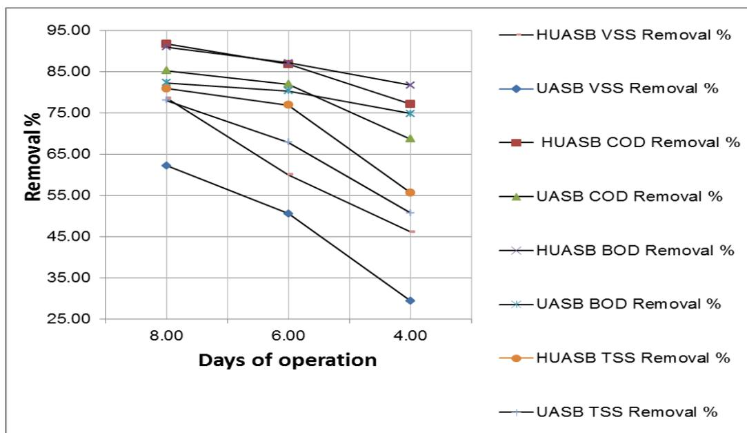
**Fig. 4:** Effect of the hydraulic detention time on the reactor s performance.
