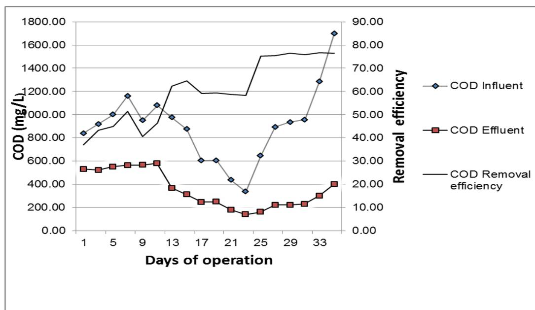
Fig. 3: COD removal efficiency of the UASB reactor during start-up period.
