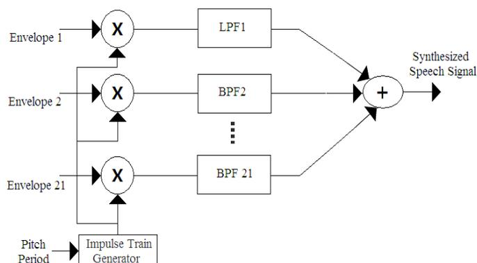
Fig. 5: Channel Vocoder Synthesizer.
