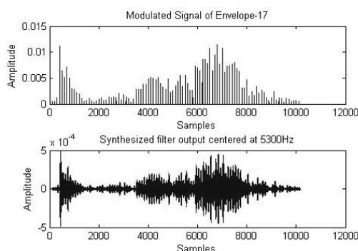
Fig. 10: (a) Waveform of modulated output of channel 16 (b) Waveform of the corresponding filtered output
