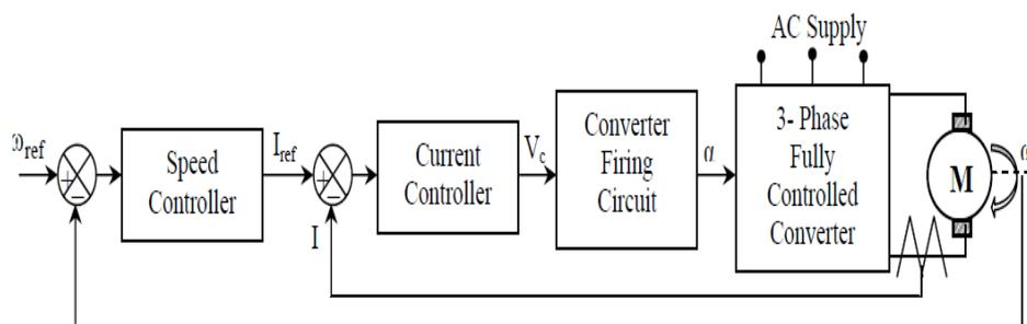
Fig. 04: Speed and current controller.
