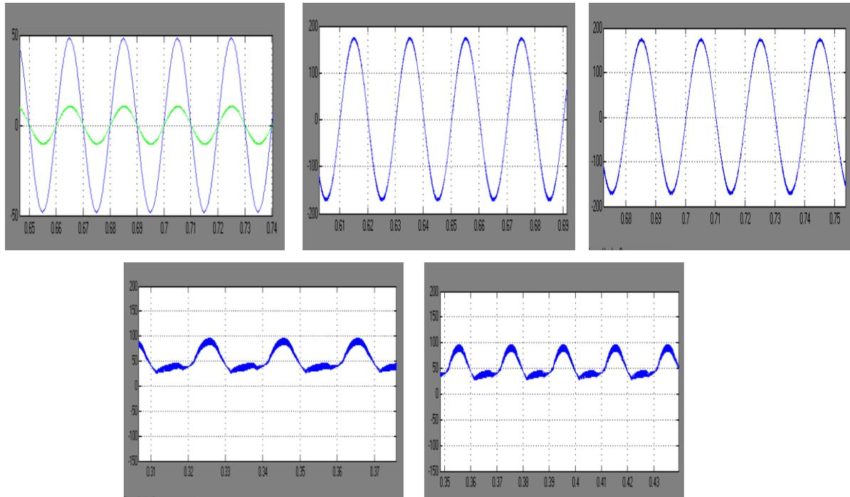
**Fig. 05:** a: Input AC voltage & current, b: Inductor current L1, c: Inductor current L2, d: Capacitor voltage C1, e: Capacitor voltage C2.
