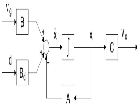
Fig. 02: State space model of Cuk converter.
