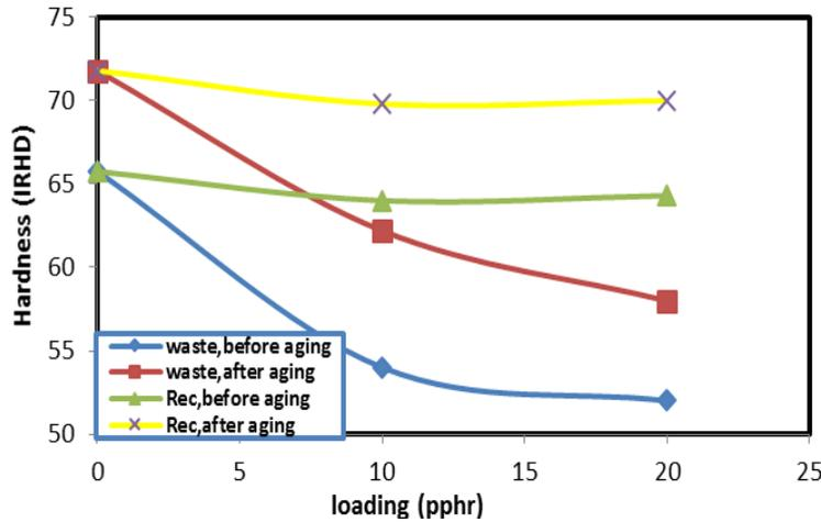
Fig. 7: Relation between hardness against waste and reclaim loading for the composite (SBR 20/NR 80). When C.B=50 pphr.
