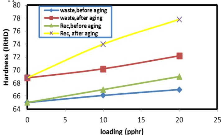
**Fig. 2:** Relation between hardness against waste and reclaim loading for the composite (SBR 60/NR 40). When C.B=50 pphr.
