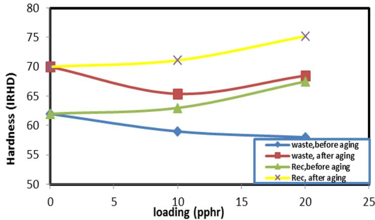
Fig. 6: Relation between hardness against waste and reclaim loading for the composite (SBR 30/NR 70). When C.B=50 pphr.
