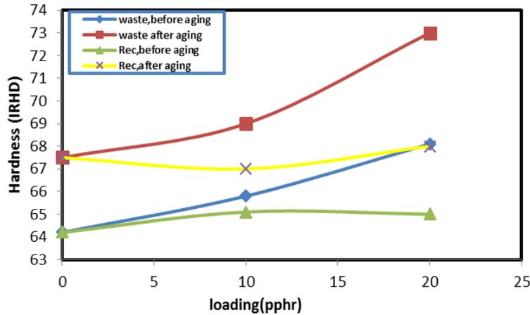
Fig. 3: Relation between hardness against waste and reclaim loading for the composite (SBR 80/NR 30/BR<sub>cis</sub>10). When C.B=50 pphr.
