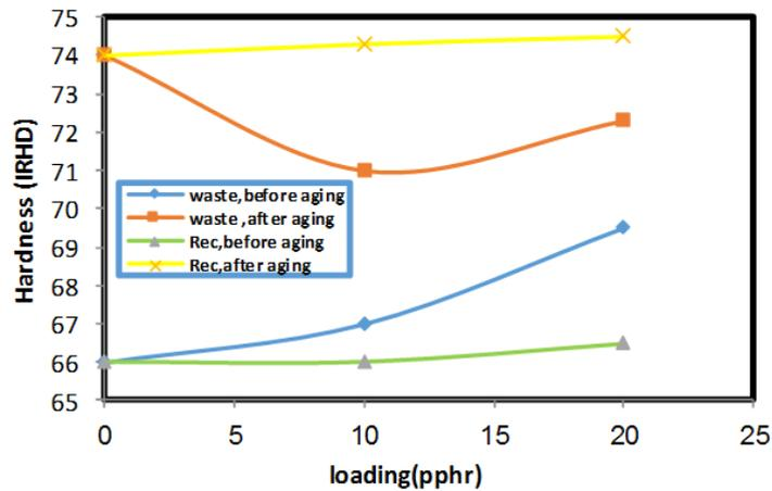
Fig. 4: Relation between hardness against waste and reclaim loading for the composite (SBR 50/NR 50). When C.B=50 pphr.
