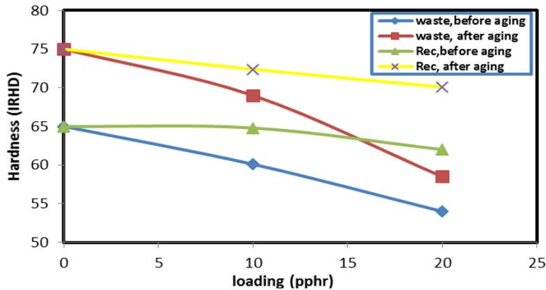
Fig. 8: Relation between hardness against waste and reclaim loading for the composite (SBR 10/NR 90). When C.B=50 pphr.
