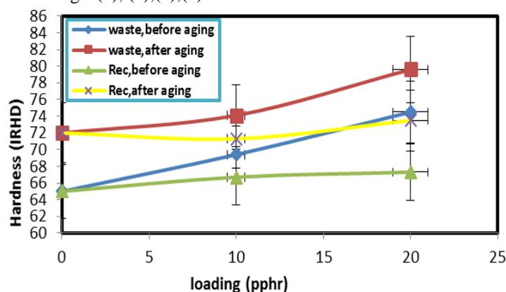
**Fig. 1:** Relation between hardness against waste and reclaim loading for the composite (SBR 80/NR 20). When C.B=50 pphr.
