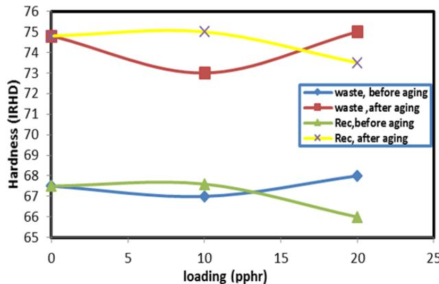
Fig. 5: Relation between hardness against waste and reclaim loading for the composite (SBR 30/NR 60/BR<sub>cis</sub>10). When C.B=50 pphr.
