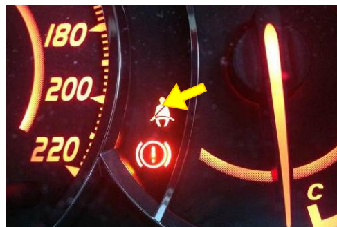
Fig. 1: An example of typical Seatbelt Reminder (SBR) on instrument panel of a passenger car
