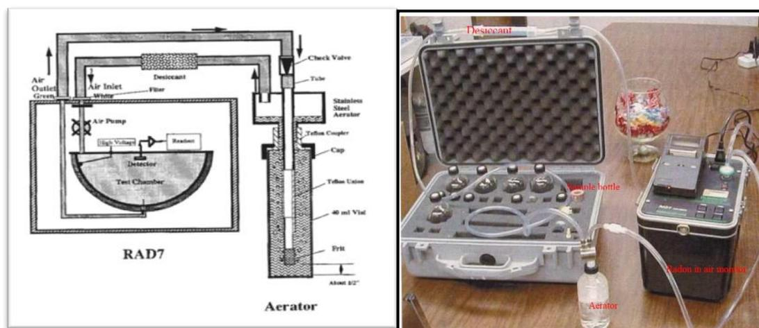
**Fig. 3:** Schematic diagram of RAD7, a solid state, ion implanted, planar Silicon alpha detector with RAD H<sub>2</sub>O assembly in (Durrige Company Inc., 2012)
