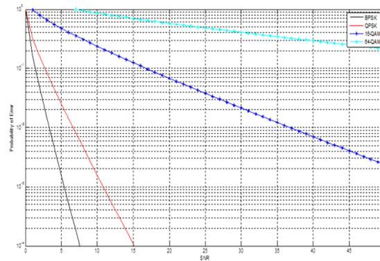
**Fig. 1:** Probability of Error (PE) for the Adaptive Modulation techniques.
