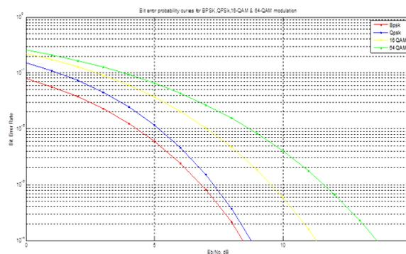
**Fig. 2:** Comparisons of modulation techniques for WIMAX via AWGN.
