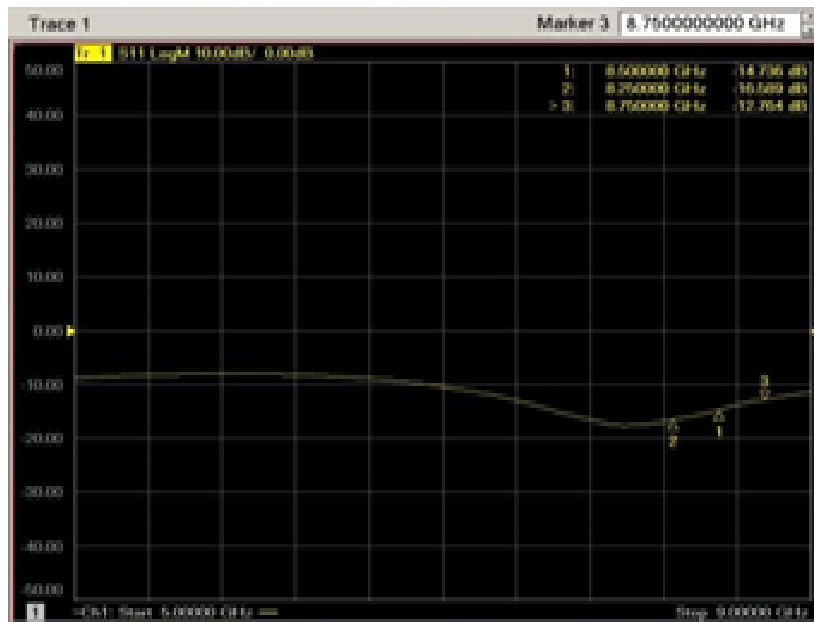
Fig. 6: Return loss of the directional monopole antenna with trapezoidal ground plane (measured by network analyzer).
