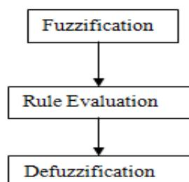
**Fig. 2:** Stage in fuzzy logic controller
