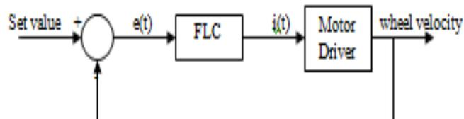
**Fig. 6:** Simple block diagram of the system
