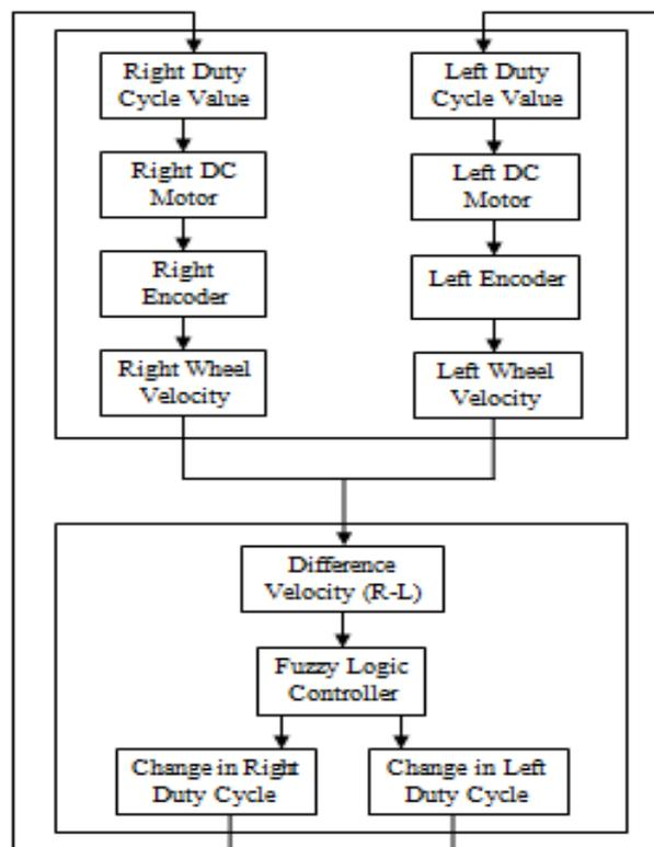
**Fig. 3:** Overall block diagram in LabVIEW program
