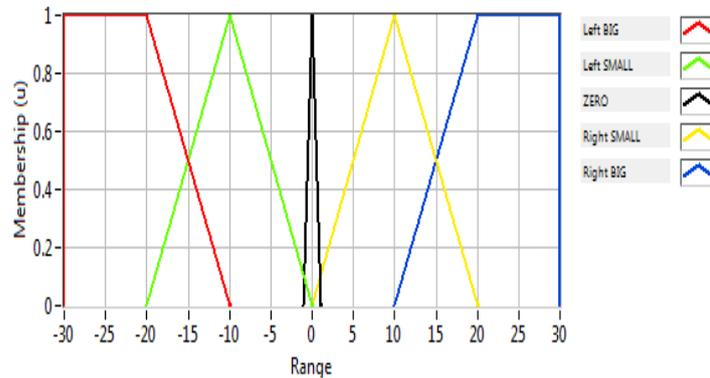
**Fig. 7:** Input variable membership functions ( $V_R - V_L$ )
