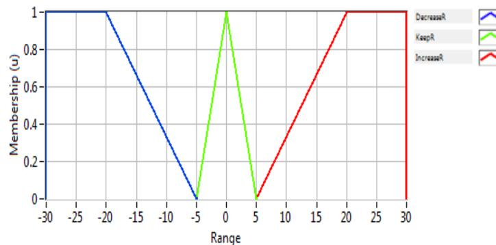
**Fig. 9 :** Output variable membership functions (DC\_Right)
