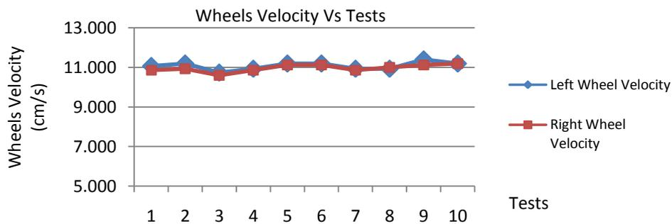
**Fig. 13:** Comparison between left wheel and right wheel velocity
