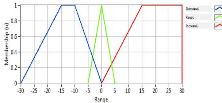
**Fig. 8:** Output variable membership functions (DC\_Left)
