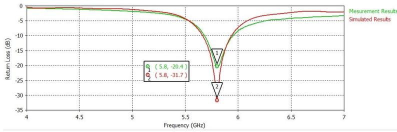
**Fig. 5:** Comparison of return loss (dB) versus frequency (GHz) of simulated and measurement of 5.8 GHz rectangular microstrip inset feed patch antenna.
