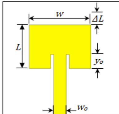
**Fig. 1:** Front view of rectangular microstrip inset feed patch antenna with the parameters dimensions indications.
