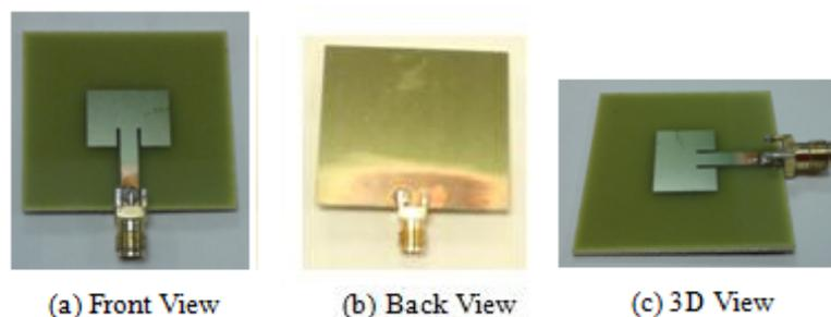
**Fig. 4:** Fabricated 5.8GHz rectangular microstrip inset feed patch antenna: (a) Front View, (b) Back View and (c) 3D View.
