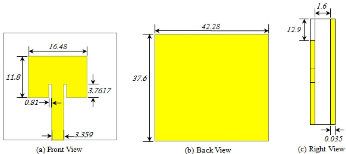
**Fig. 3:** Final CST software simulated design dimension (mm) of rectangular microstrip inset feed patch antenna: (a) Front View, (b) Back View and (c) Right View.
