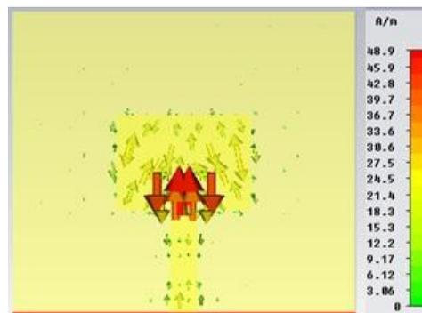
**Fig. 8:** Simulated surface current density (A/m) for 5.8 GHz rectangular microstrip inset feed patch antenna.
