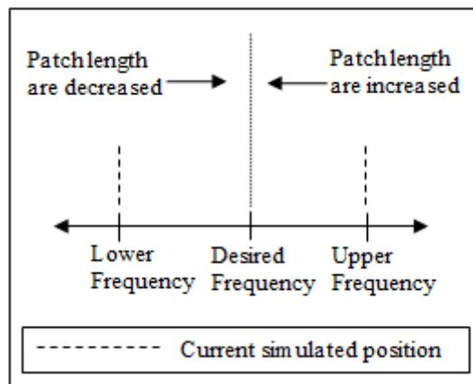
**Fig. 2:** Parameter study of patch length variation to frequency shift.
