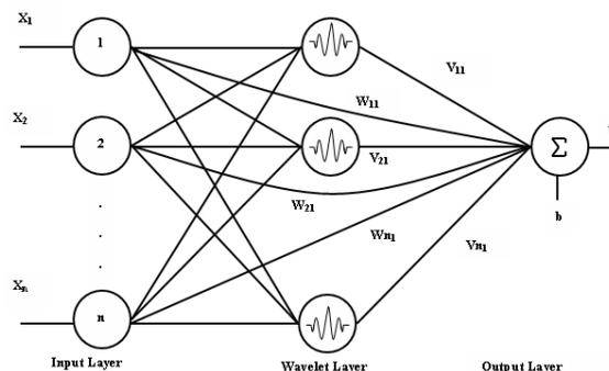
Fig. 4: Typical architecture of a MWNN.
