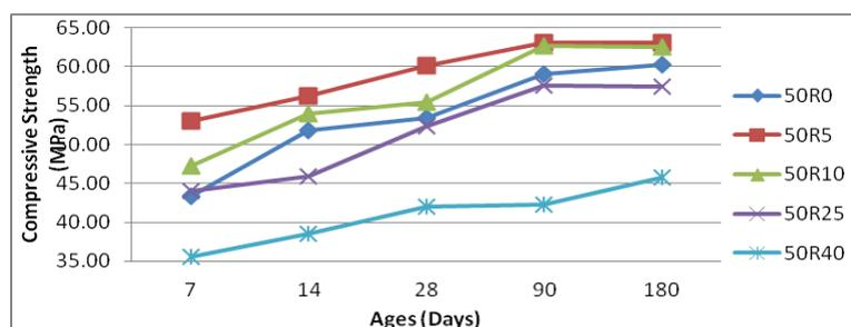
Fig. 3.1: Compressive Strength Of Specimen Concrete Grade 50 Versus Ages.
