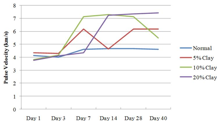
**Fig. 4:** Pulse velocity concrete between four sample specimens.
