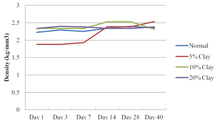
Fig. 1: Density concrete between four sample specimens.
