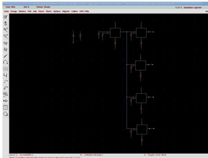
Fig. 2: Experimental setup for measuring leakage current (a) of basic gates with varying fanout in cadence virtuoso.
