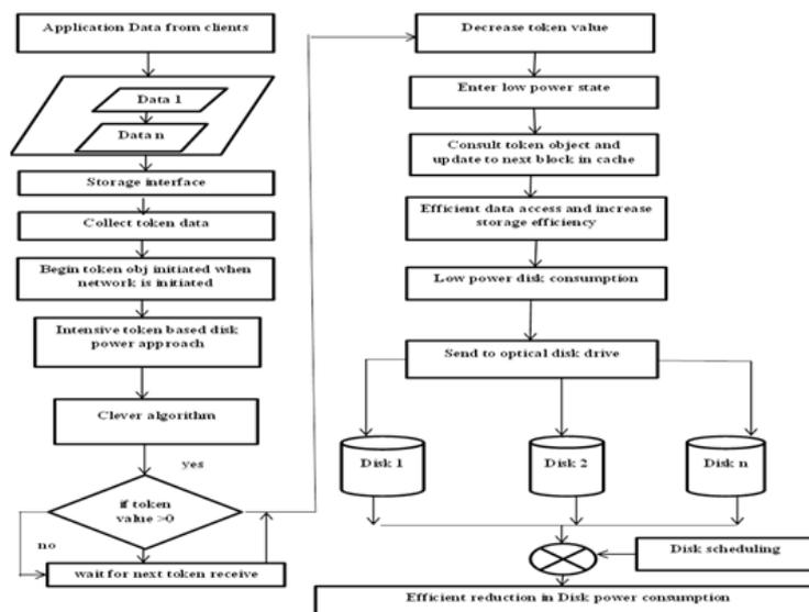
**Fig. 2:** Intensive token based disk power approach by using clever algorithm.
