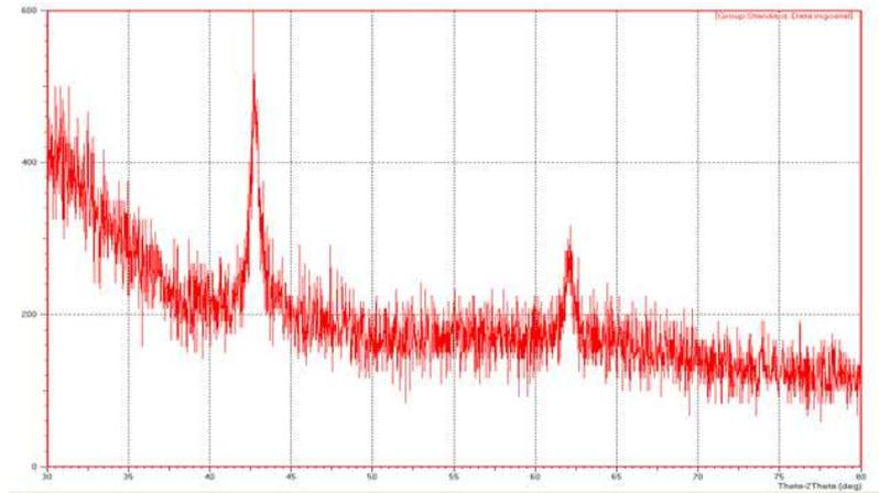
**Fig. 1.a** XRD of MgO NPs prepared by PLAL method
