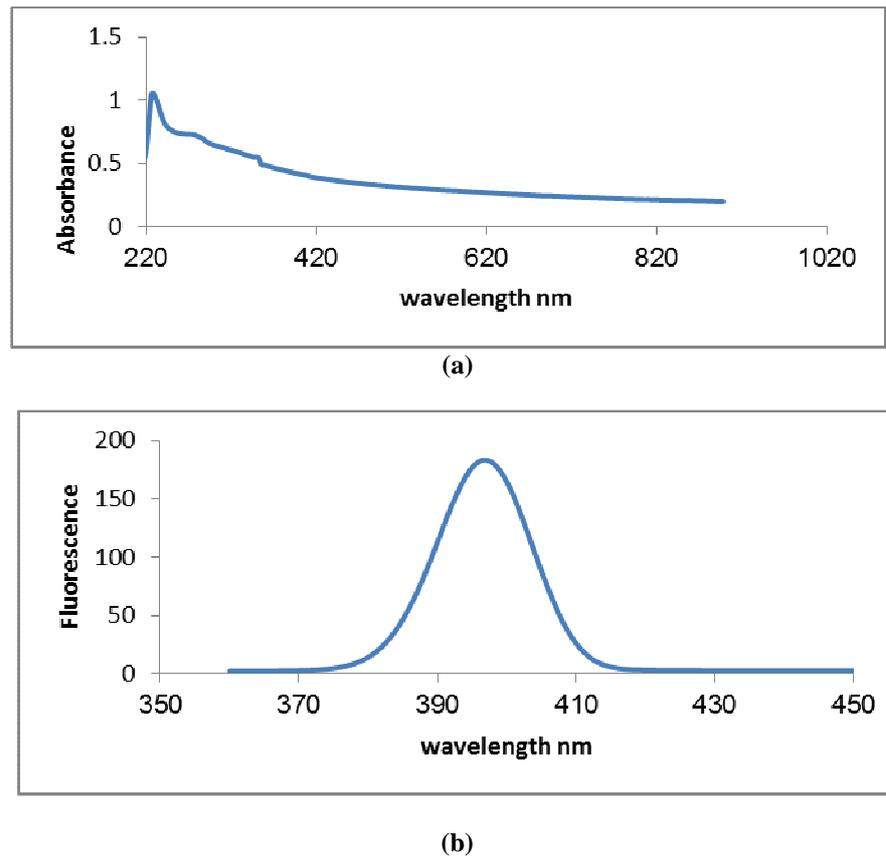
**Fig. 5:** Absorbance (a) and Fluorescence (b) spectra of MgO NPs prepared chemical method
