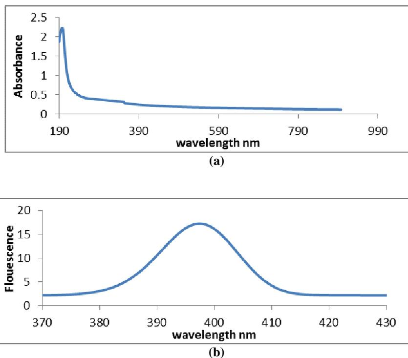
**Fig. 4:** Absorbance (a) and Fluorescence (b) spectra of MgO NPs prepared by PLAL method
