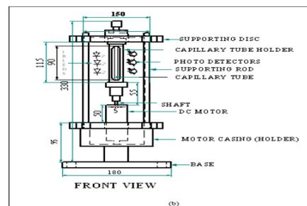
**Fig. 1b:** Front view of the Separation part mechanical assembly.
