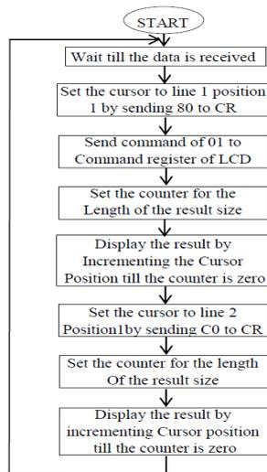
Fig. 4: b) Flow chart of LCD.
