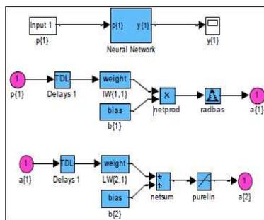
Fig. 6: RBF Simulink model for classification.
