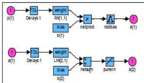
Fig. 5: Hidden and output layer of RBF.
