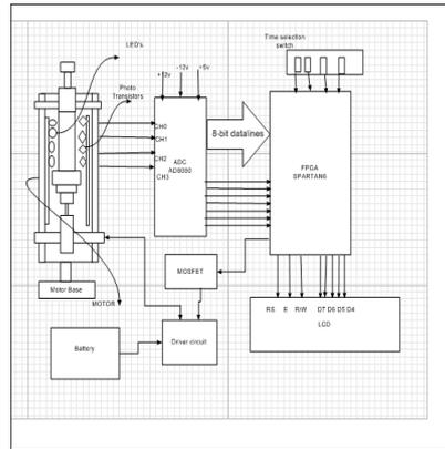
**Fig. 2:** Circuit diagram of the FPGA based instrumentation System.
