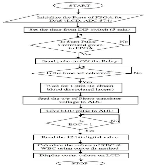
Fig. 4: A Flow chart of the instrumentation System.
