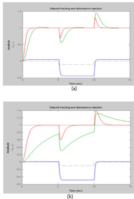
Fig. 3.3: Load disturbance factor using (a) Existing PI-LFL Controller (b) PID-RNF Controller.
