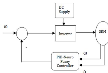
Fig. 2.1: Block Diagram of SRM speed control using RNF.
