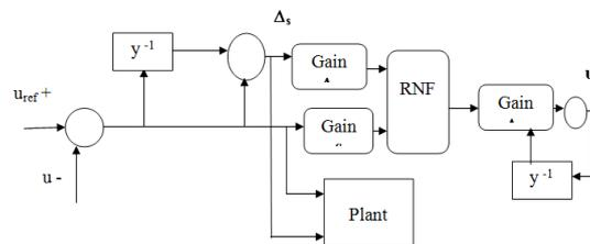
Fig. 2.2: Block Diagram of Reconciling Neuro-Fuzzy Controller.
