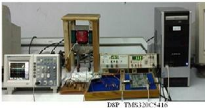
Fig. 15: Experimental set up for Synchronous demodulation method (digital).
