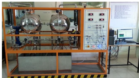
Fig. 3: Experimental set up of coupled spherical tank system.
