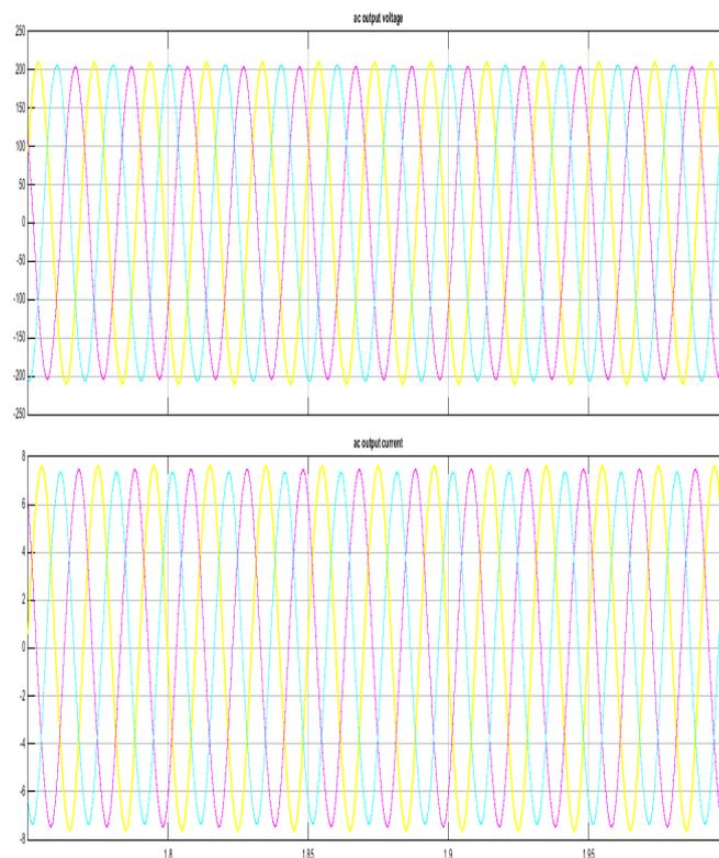
**Fig. 10:** Simulation results of phase peak inverter output voltage and current
