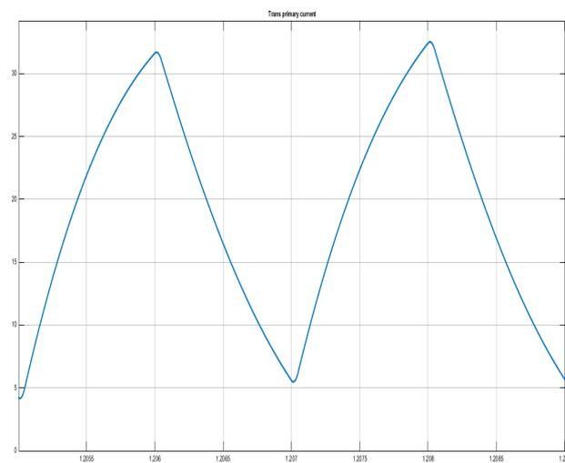
**Fig. 9:** Simulated transformer primary current
