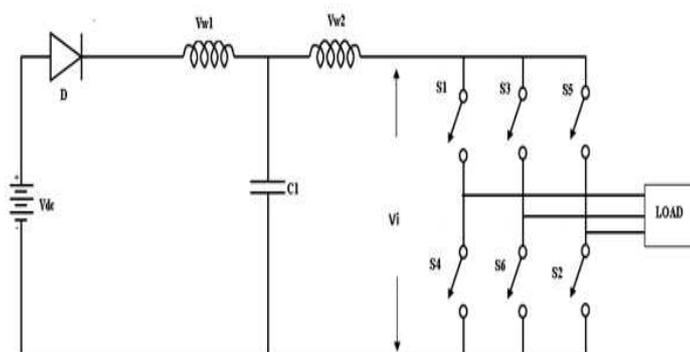
**Fig. 2:** Trans Z-source inverter
