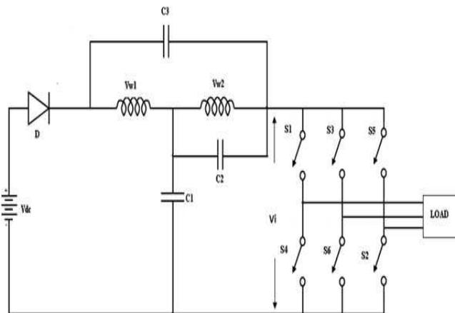
**Fig. 3:** Proposed Coupled Capacitor Trans Z Source Inverter
