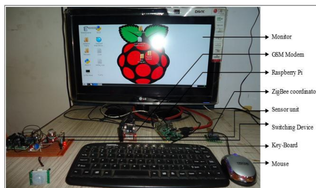
Fig. 9: Working Experimental setup. (a) Wireless sensing unit responding to E-mail with subject 'ON1' i.e.
