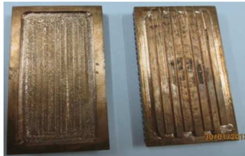
Fig. 3: Interior details of the fabricated minichannel evaporator.
