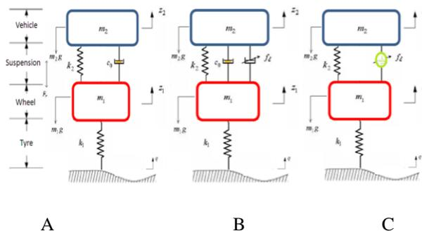
**Fig. 2:** (a) Passive, (b) Semi-active and (c) Active suspension system.
