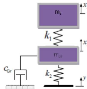
**Fig. 3:** A schematic of the Groundhook control system.
