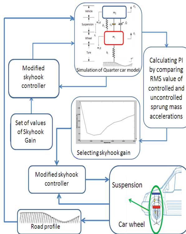
**Fig. 5:** Schematic of the suspension systems based on proposed modified skyhook control system with adaptive skyhook gain.
