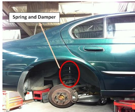
**Fig.1:** Rear suspension system without wheel of a vehicle.
