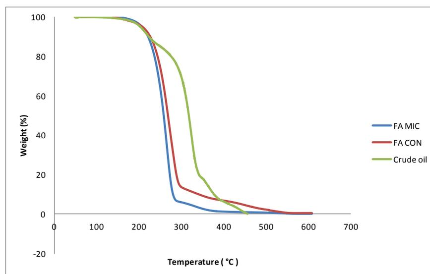
**Fig. 2:** Thermogravimetric curves for Fatty acids microwave, Fatty acids conventional and crude oil.
