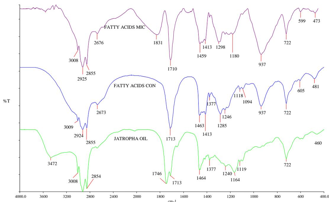
**Fig. 3:** Comparison of FTIR spectra for fatty acids of microwave, fatty acids conventional and jatropa oil.
