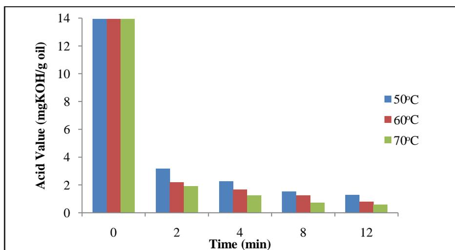
**Fig. 2:** Influence of temperature and reaction time on reduction of acid value in *Ceiba Pentandra* Seed Oil.
