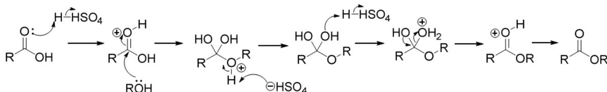
Fig. 1: Mechanism for esterification reaction (Loudon, 2009).
