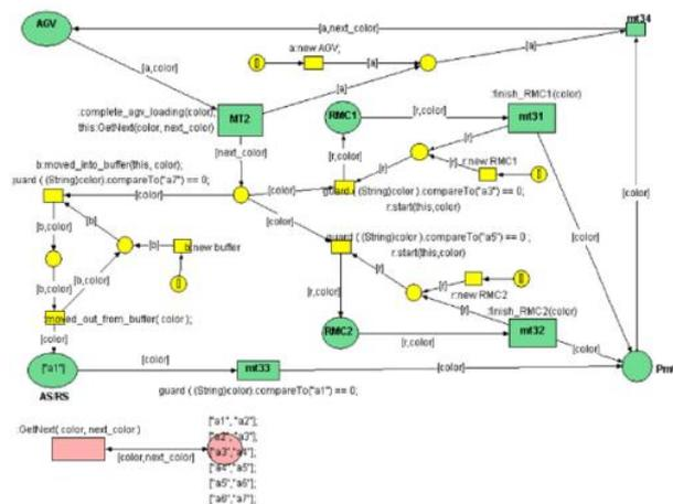
Fig. 2: System level Petri net model of RMS (Xiuli, M., 2010).
