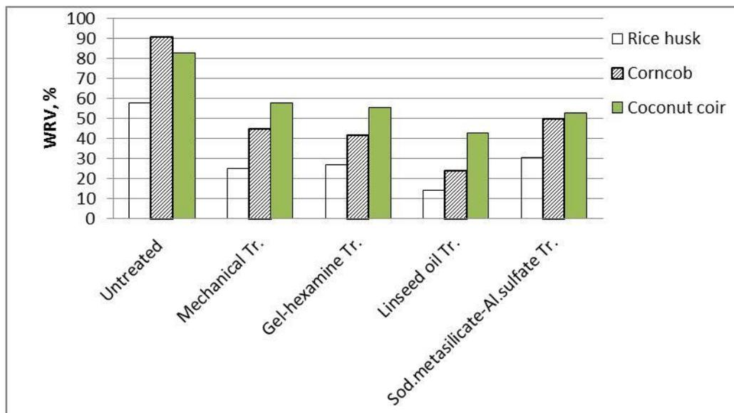
**Fig. 2:** Comparison between the WRV % of untreated and treated fibers.
