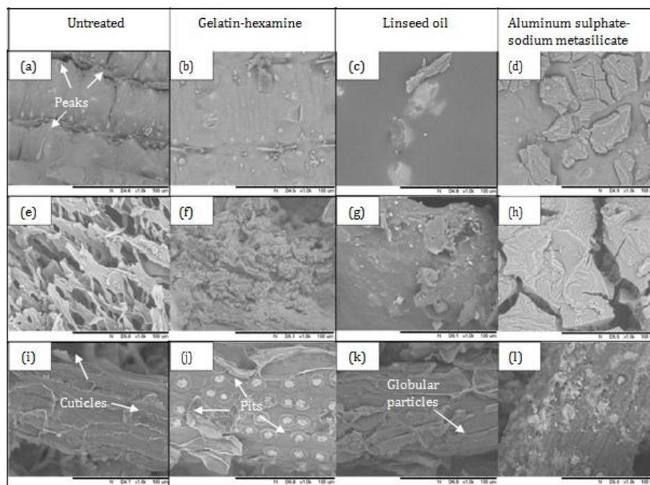
**Fig. 1:** SEM micrographs of fibers: (a-d) untreated rice husk fiber, gelatin-hexamine treatment, linseed oil treatment, and sodium metasilicate-aluminum sulphate treatment respectively, (e-h) untreated corncob fiber, gelatin-hexamine treatment, linseed oil treatment, and sodium metasilicate-aluminum sulphate treatment respectively, (i-l) untreated coconut coir fiber, gelatin-hexamine treatment, linseed oil treatment, and sodium metasilicate-aluminum sulphate treatment respectively.
