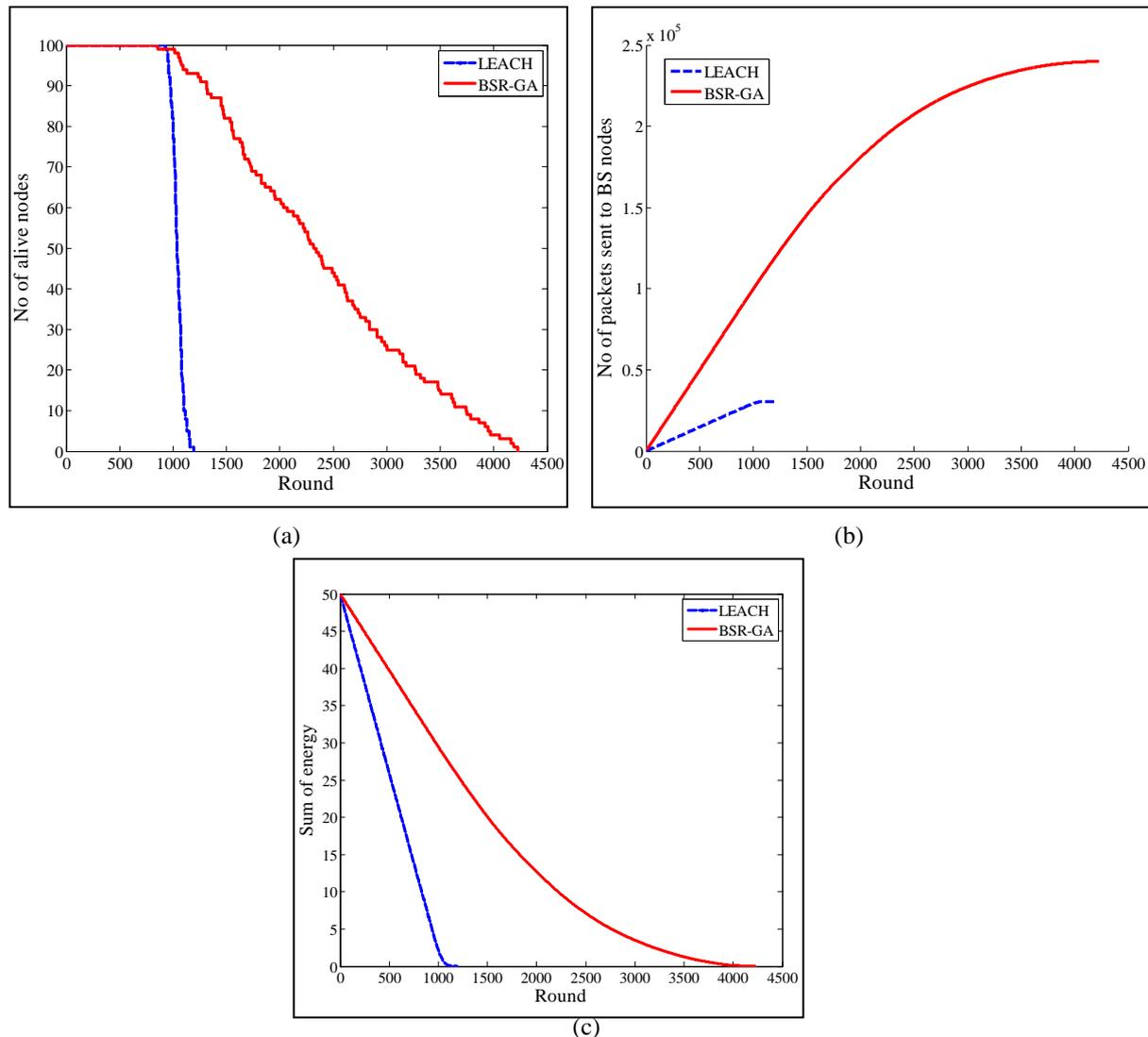
**Fig. 3:** (a) Number of nodes alive over round for network field. (b) Sum of energy over round. (c) Number of packets data sent to BS over round.
