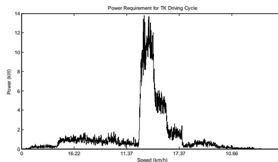
**Fig. 5:** PHERB power requirements for TK driving cycle.
