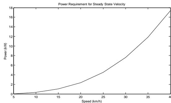
**Fig. 2:** PHERB power requirements for steady state velocity.
