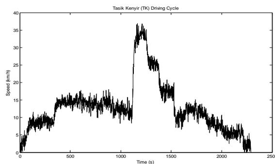
**Fig. 4:** The TK driving cycle.
