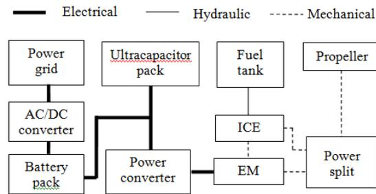
**Fig. 1:** A schematic illustration of the proposed series-parallel PHERB powertrain.
