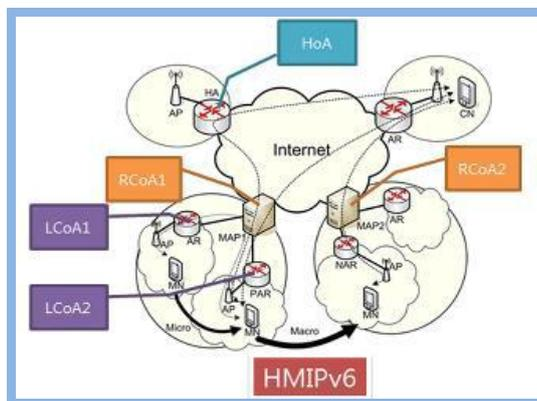
**Fig. 3:** Network Diagram of HMIPv6.
