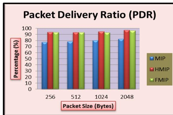
Fig. 8: Comparison Chart of Packet Delivery Ratio (PDR).
