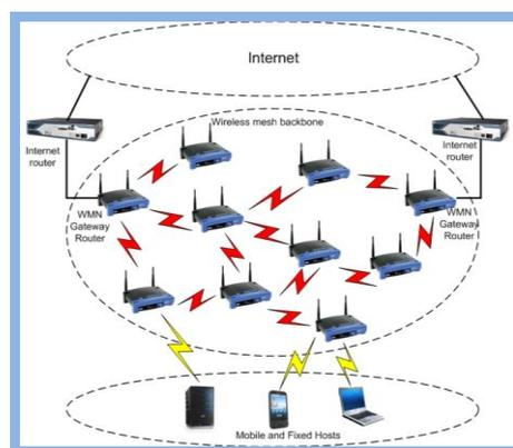
**Fig. 5:** Wireless Mesh Network Diagram.
