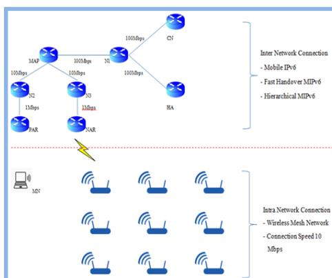
**Fig 6:** Inter & Intra Network Connection Diagram.
