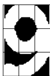
Fig. 5: Zone-Based Directional Pixel density from all sides of bounding box
