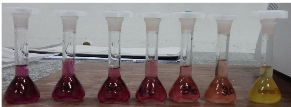
Fig. 6: Calibration curve color from Alizarin samples with different concentrations.
