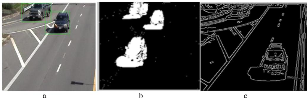
**Fig. 2 a:** Tracked vehicle, b. Background subtraction c. Boundary extraction
