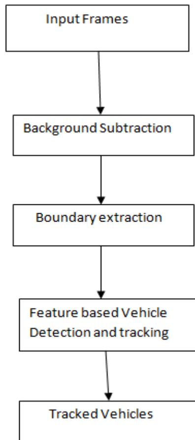
**Fig. 1:** Vehicle Detection and Tracking System
