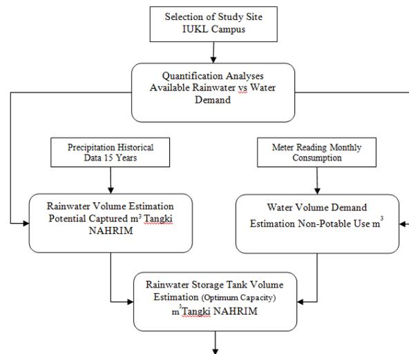
**Fig. 1:** conceptual framework for assessing RWH installation at the IUKL campus site.
