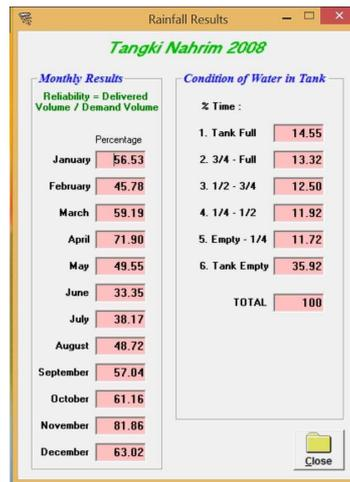
Fig. 5: Monthly reliability and tank status when tank size 25m<sup>3</sup>.
