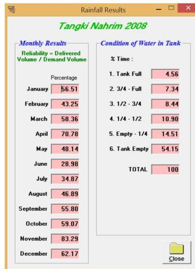
**Fig. 8:** Monthly reliability and tank status when tank size 75m<sup>3</sup>.
