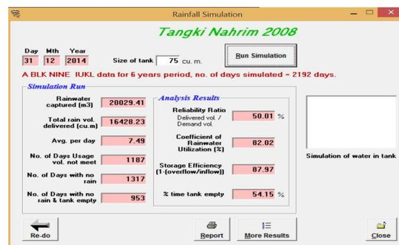
Fig. 7: Tanki NAHRIM output data, reports the total captured rainwater based on the roof dimension and the precipitation data, total delivered rainwater based on the rainwater data profile and selected tank size, average daily availability, reliability ratio, rainwater utilization percentage, and storage efficiency based on selected tank size.
