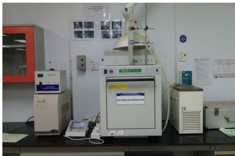
Fig. 1: Experimental Set-up of Milestone Ethos Microwave Extraction System
