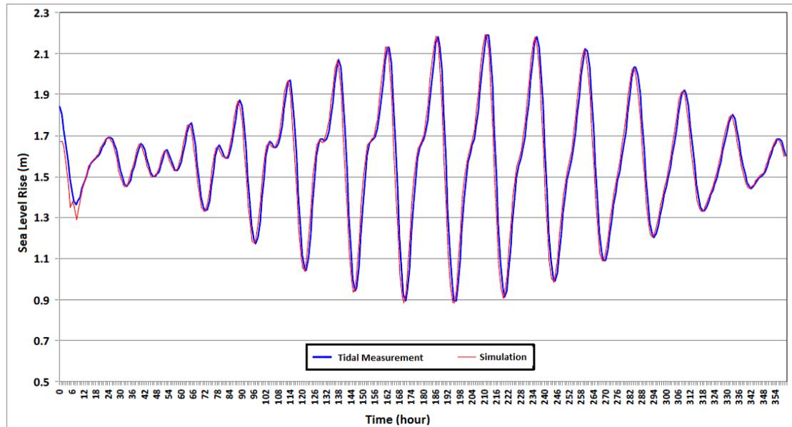
**Fig. 3:** Comparison of water level simulation results with measurements for 15 days in the waters of Makassar Beach at 119° 21' 49,50"BT and 5° 11' 56,35"LS. (Source: Arifin *et al.*, 2012)
