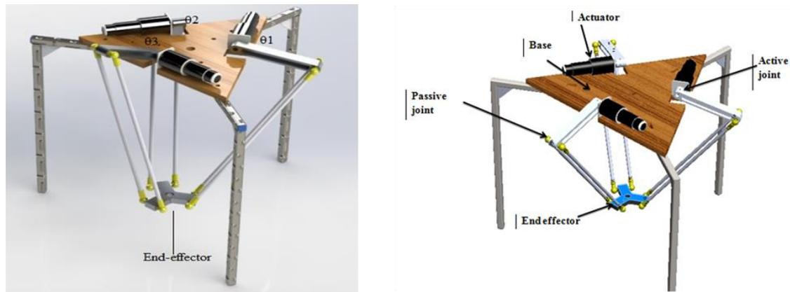
**Fig. 1:** 3D CAD model for delta robot
