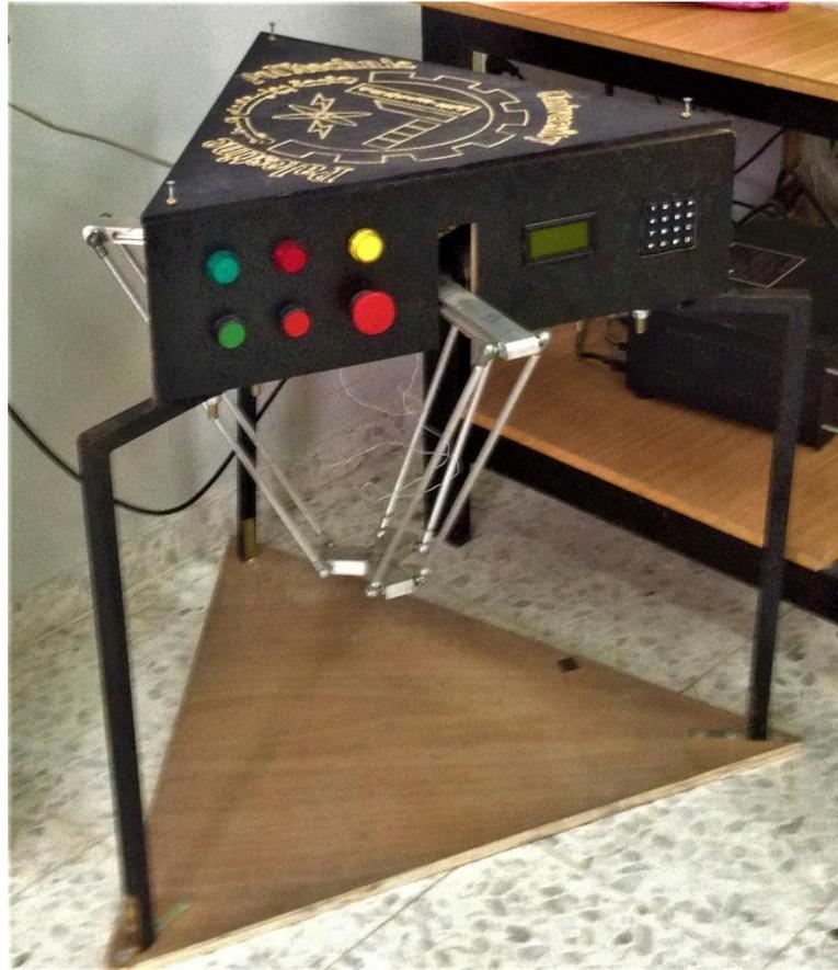
**Fig. 9:** Real Design for 3DOF Delta Robot at PPU
