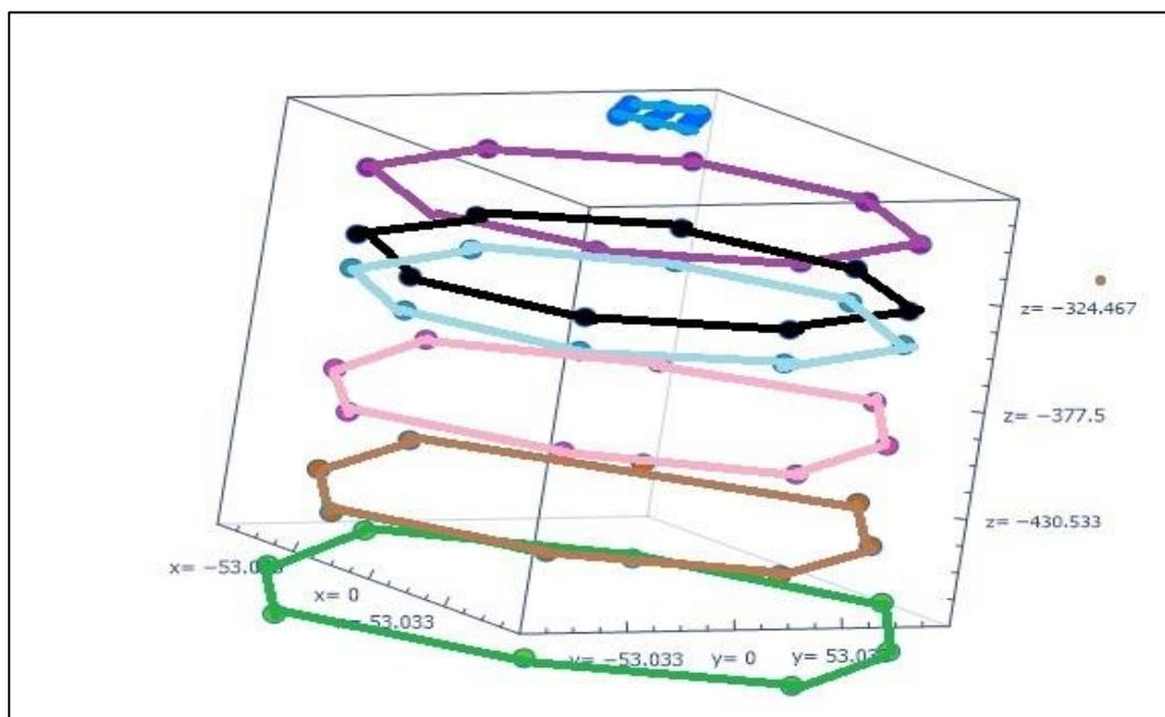
**Fig. 10:** Workspace of delta robot in xyz directions
