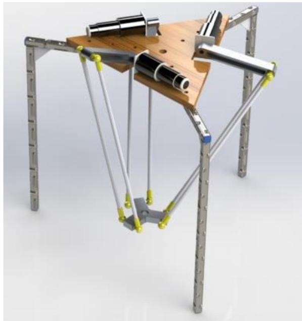
**Fig. 8:** Delta robot after assembly
