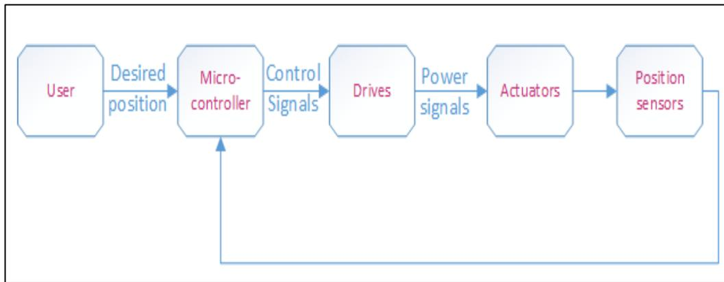
**Fig. 11:** Overall control block diagram for delta robot
