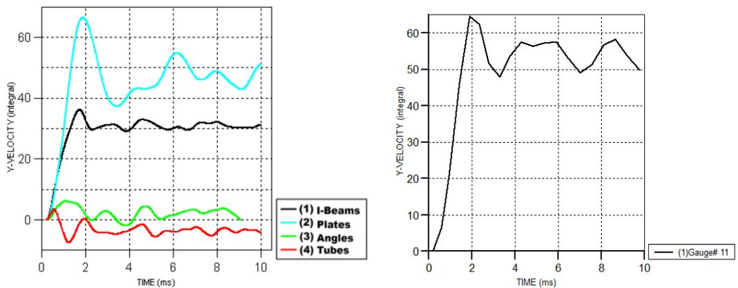
Fig. 4: Deformation time history at gauge no.11
