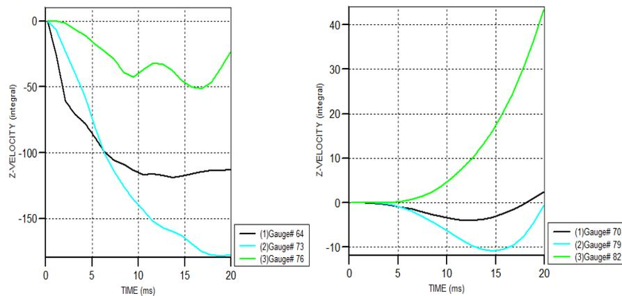
**Fig. 11:** deformation time history for front and rear plate
