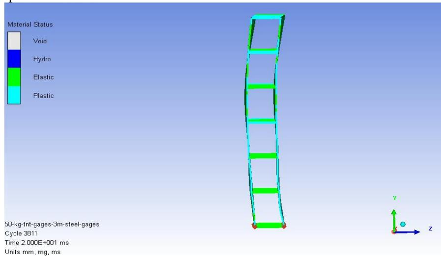
Fig. 19: Location of the maximum deformation located at the panel middle.
