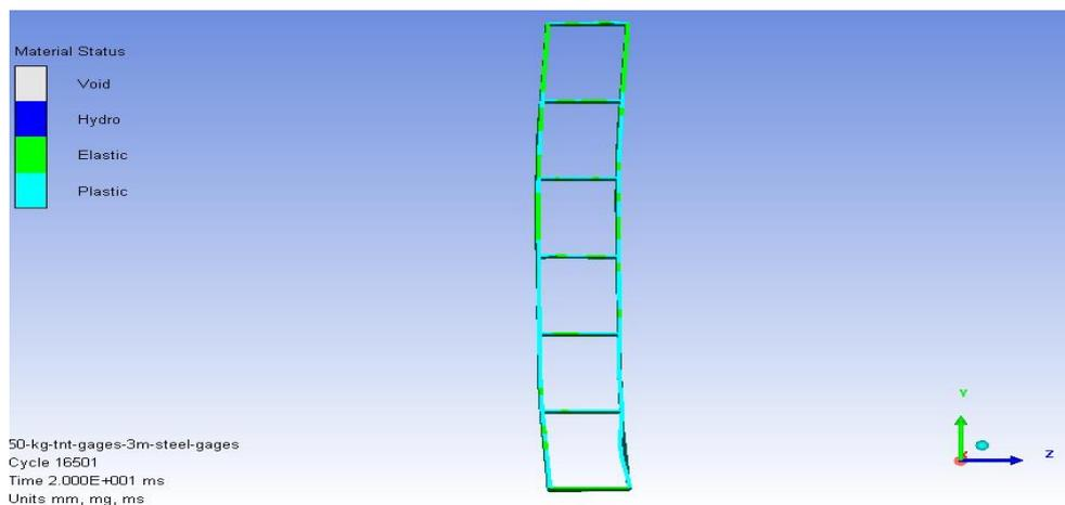
**Fig. 22:** Location of the maximum deformation located at the panel middle.
