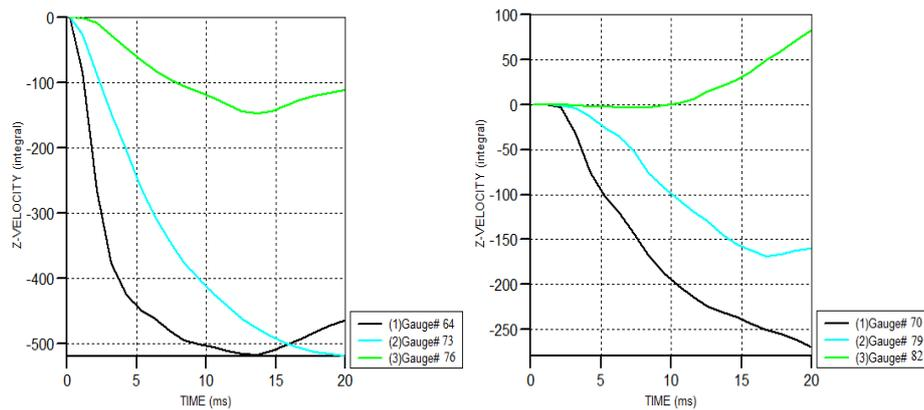
**Fig. 8:** deformation time history for front and rear plate
