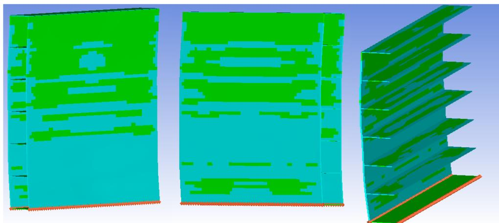
**Fig. 24:** Plastic deformation region in front, rear and horizontal plate.
