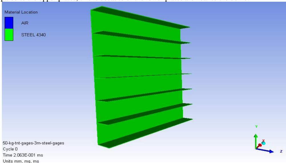
**Fig. 21:** Orientation of horizontal plates inside the panel.
