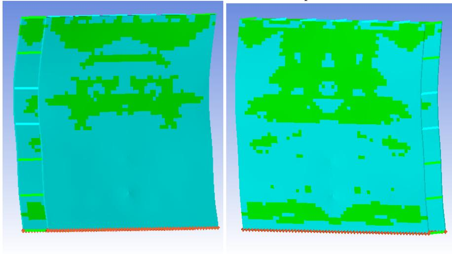
Fig. 20: Plastic deformation region in front and rear plate.
