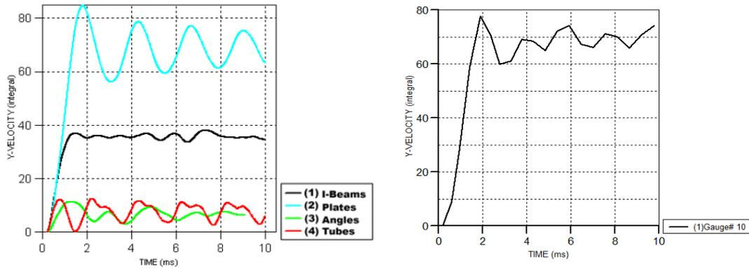
Fig. 3: Deformation time history at gauge no.10
