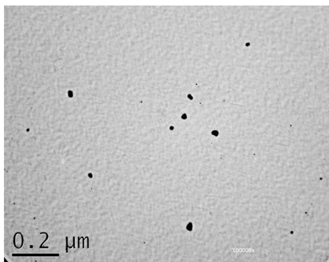
**Plate 3.2:** Representative TEM micrograph silver nanoplates synthesize by the reduction of  $\text{AgNO}_3$  ions in a *Jania rubens* ethanolic extract.
