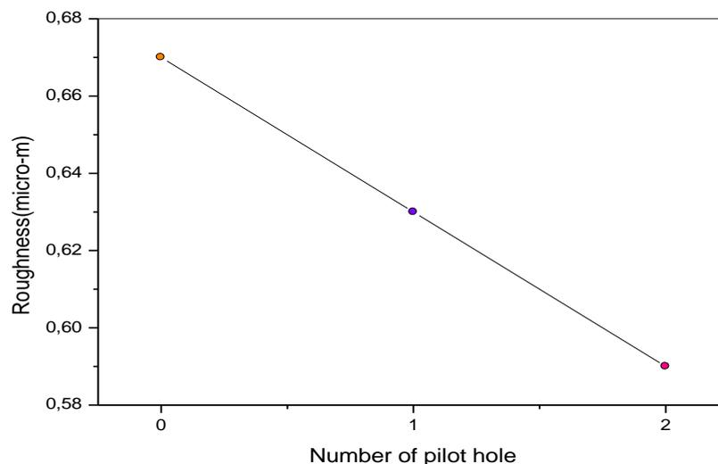
**Fig. 10:** Roughness values of drilled holes with and without pilot hole
