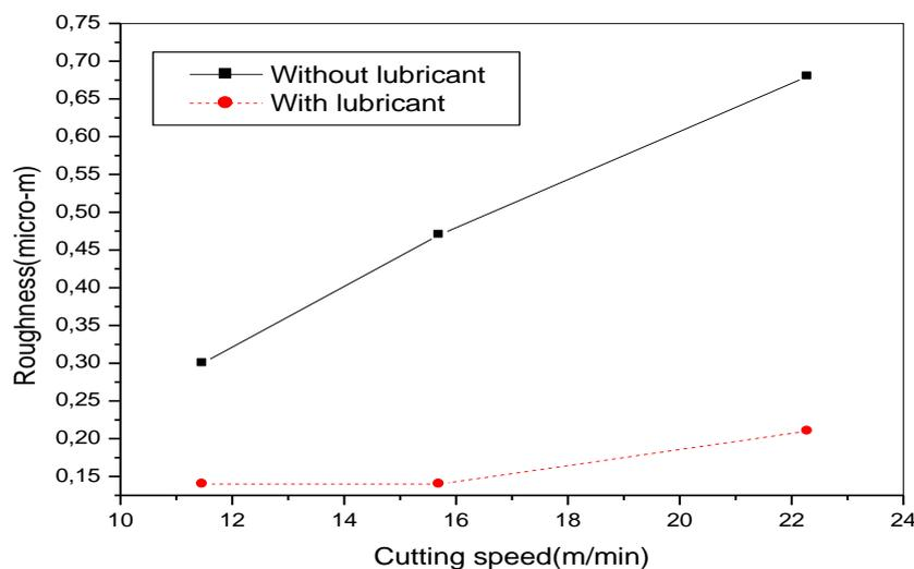
**Fig. 9:** Comparison of the surface roughness (with and without lubricant).
