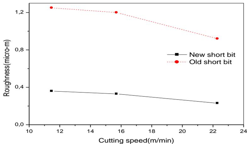
**Fig. 7:** Comparison of the surface roughness (new and worn bit)
