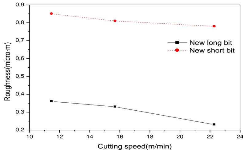
**Fig. 8:** Comparison of the surface roughness (short and long bit)
