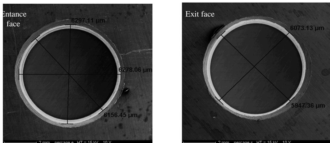
**Fig. 5:** Entrance and exit diameters measurement (SEM)
