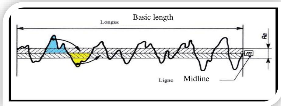
**Fig. 2:** Average arithmetic deviation "Ra".
