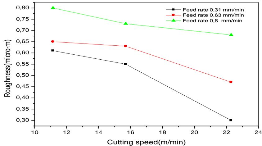
**Fig. 6:** Roughness variation according to the cutting speed and to the feed rate.
