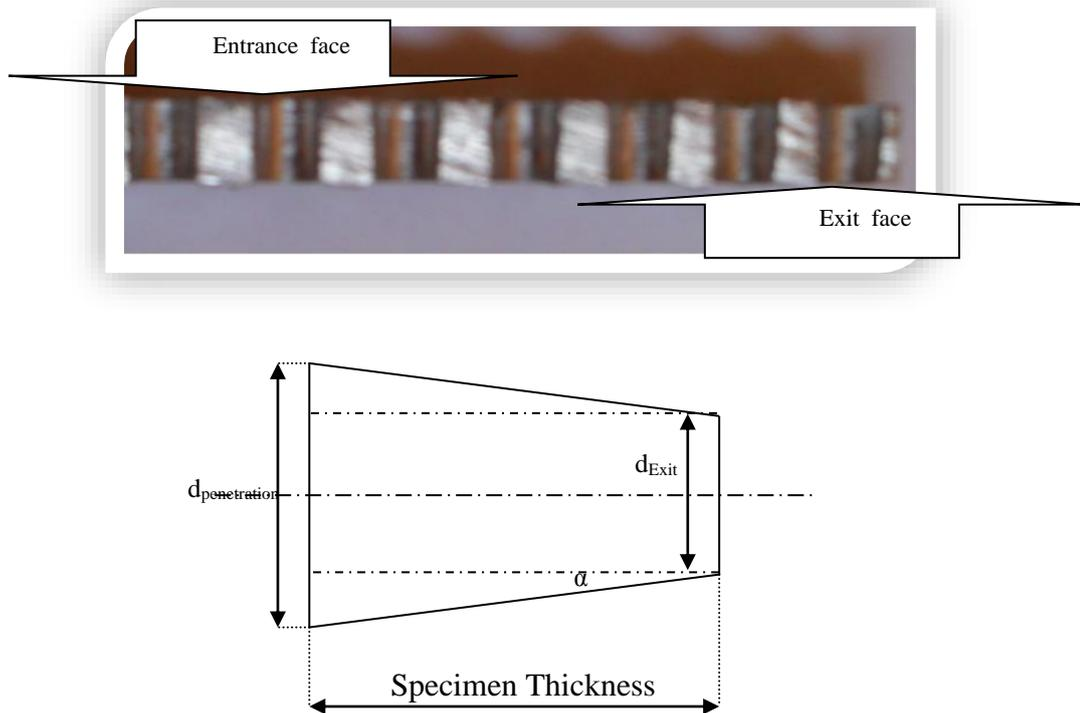
**Fig. 4:** Holes conicality
